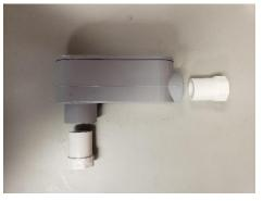
3. Screw the PG9 connectors into the 3/8 adapters. Tighten by hand.
