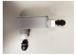
4. Prepare the valve and junction box for attachment by cleaning the side of the valve (see picture) and the inside of the junction box with isopropyl alcohol.
