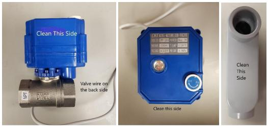
5. When alcohol is dry put two strips of 3M VHB Tape on the horizontal of the of the valve (see picture). Rub tape back and forth to ensure any air bubbles are pushed out.
